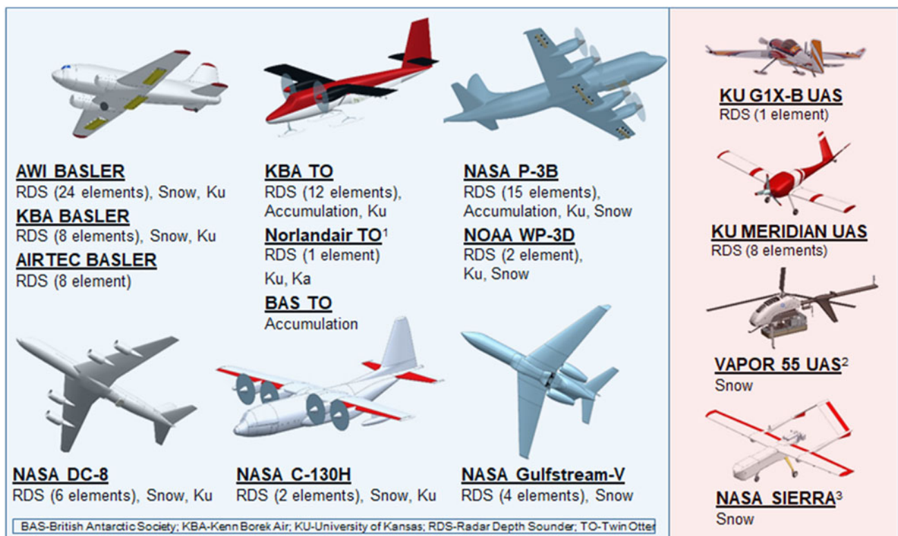
Fig. 1. Overview of aircraft that have been used to fly CReSIS radars. Each platform's radar configuration is listed below the vehicle and the number of antenna elements in the RDS array is indicated in the parentheses. 1 The RDS and Ku and Ka are two separate configurations; 2 Radar system has been developed, but has not yet been flown for a mission. 3 Radar system integrated on the vehicle, but never flown due to loss of the vehicle.
