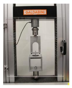
Figure 12. Test setup of the pull-out test.
