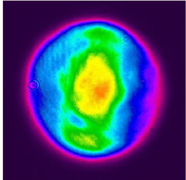
**Figure 9.** Near-field beam profile of the amplified pulse.
