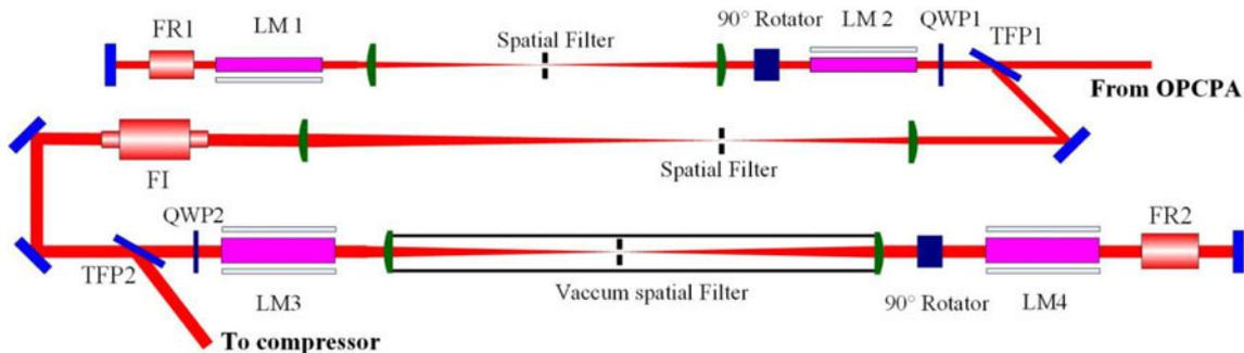
**Figure 8.** Layout of the two Nd:glass rod amplifiers. TFP1, TFP2: thin film polarizer; QWP1, QWP2: quarter wave plate; LM1, LM2: single-flashlamp-pumped Nd:glass rod module; FR1, FR2: Faraday Rotator; FI: Faraday Isolator; LM3, LM4: double-flashlamp-pumped Nd:glass rod module.
