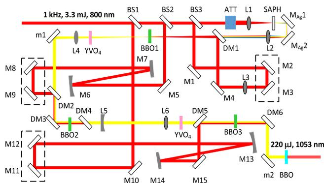
Figure 2. Layout of the OPA-SHG pulse cleaning device. BS1–BS3: beam splitter; ATT: attenuator; L1–L6: lens; SAPH: sapphire plate;  $M_{Ag1}$ ,  $M_{Ag2}$ : silver mirror; DM1–DM6: dichroic mirror; M1–M15: 800 nm HR mirror; m1, m2: 2106 nm HR mirror.
