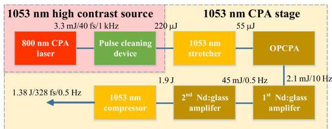
Figure 1. Schematic overview of the double CPA laser system.
