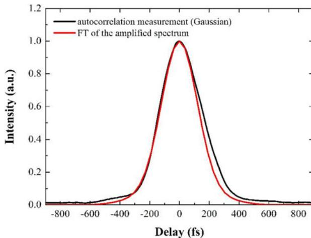
**Figure 10.** Autocorrelation measurement and Fourier-transform-limited pulse duration.
