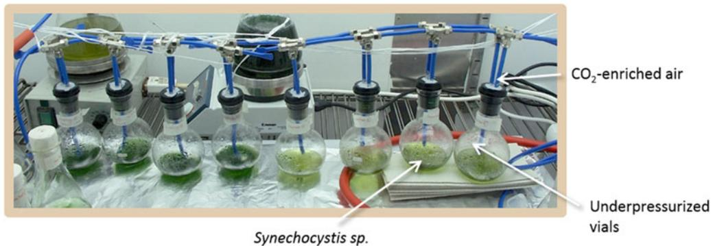
**Fig. 5.** Underpressurized culture vials used in Kirsi Lehto's laboratory (at the University of Turku, Finland) to grow cyanobacteria in low-pressure/high pCO<sub>2</sub> atmospheres.
