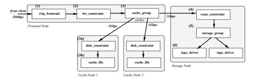
Fig. 2. Sample deployment of a VoDKA configuration.
