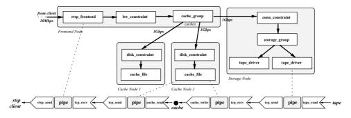
Fig. 7. Chaining of pipes in a transmision.
