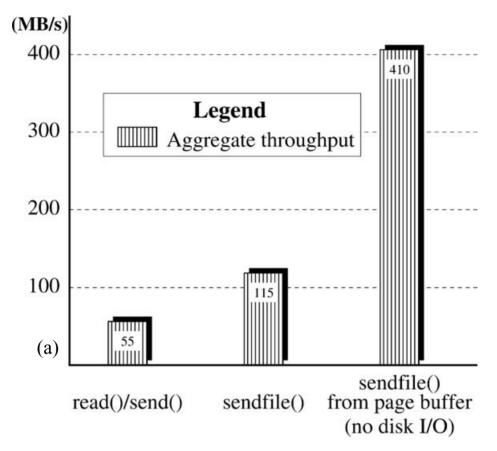
Fig. 11(a). Throughput comparison using different interfaces.
