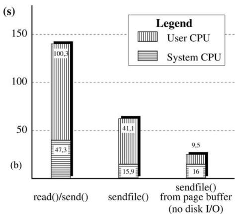
Fig. 11(b). CPU usage comparison with different interfaces.
