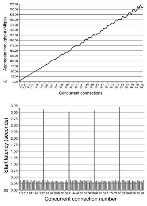
Fig. 10. (a) Aggregate bandwidth in a cluster. (b) Latency when starting connections in a cluster.
