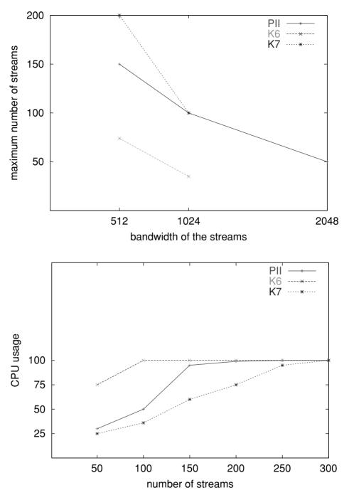
Fig. 9. Maximum number of streams and CPU usage for each of the servers.
