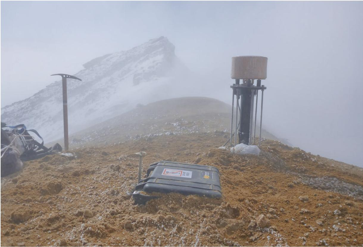
**Fig. 4.** The Seebeck generator installed in the hot ground. The data logger is housed in the black Peli case.
