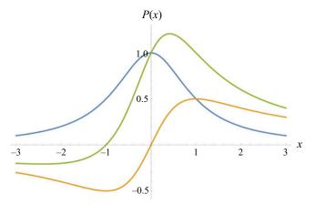
FIGURE 2. Dipole-type pressure impulses P(x): the symmetric case where P(x) = P(-x) is represented by (A = 1, B = 0). The antisymmetric case where P(x) = -P(-x) is represented (A = 0, B = 1). An asymmetric case (A = B = 1) is added.
