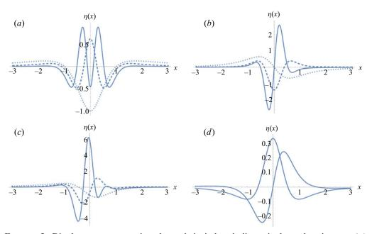
FIGURE 3. Dipole-type pressure impulses: their induced dimensionless elevations:  $\eta_1(x)$  (dotted),  $\eta_2(x)$  (dashed),  $\eta_3(x)|_{G=0}$ . (a) The symmetric case A=1, B=0. (b) The antisymmetric case A=0, B=1. (c) An asymmetric case A=B=1. (d) Gravitational contributions  $\eta_3/G$  for A=1, B=0 (symmetric) and A=0, B=1 (antisymmetric).
