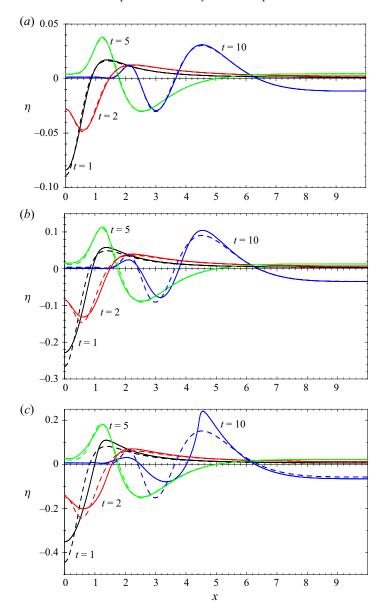
FIGURE 6. Snapshots for different times with an initial pressure as (9.4) with  $P_0 = 0.1$ , 0.3, 0.5 (a–c). Dashed lines are computed with the linearized set of (9.1), (9.2), solid lines correspond to fully nonlinear solutions. Nonlinear effects increase with increasing initial pressure and surface amplitude.
