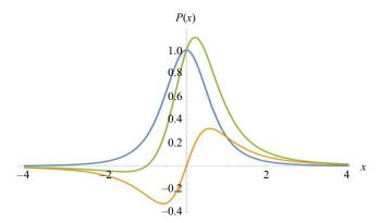
FIGURE 4. Quadrupole-type pressure impulses P(x): the symmetric case where P(x) = P(-x) is represented by (A = 1, B = 0). The antisymmetric case where P(x) = -P(-x) is represented (A = 0, B = 1). An asymmetric case (A = B = 1) is added.
