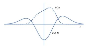
FIGURE 1. Definition sketch for a two-dimensional free-surface flow generated by a surface pressure impulse P(x) (dashed) on an initially horizontal surface. The surface elevation is  $\eta(x,t)$ .
