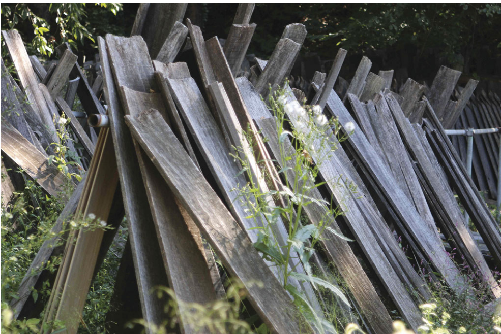
Figure 3. Paulownia wood for kayagŭm zither soundboards, drying, behind Ko Hŭnggon’s workshop, 2014 (photo by Keith Howard; all rights reserved).
