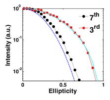
**Figure 4.** Measured dependences of 7th (black circles) and 3rd (red squares) harmonic signals from excited argon atoms on the elliptical polarization of the probe pulse. The green solid and blue dotted curves represent the theoretical predictions.
