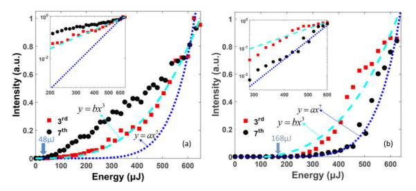
Figure 3. (a) Measured 7th (black circles) and 3rd (red squares) harmonic signals from excited argon atoms as a function of the probe pulse energy; (b) measured 7th and 3rd harmonic signals from unexcited argon atoms as a function of the probe laser energy. The green dashed and blue dotted curves are the corresponding fitting curves with function  $I^q$ , where q is the harmonic order. Inserts: measured harmonic signals as a function of the probe laser energies with logarithmic scales.
