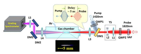
Figure 1. Schematic diagram of the experimental setup. TS: telescope system.
