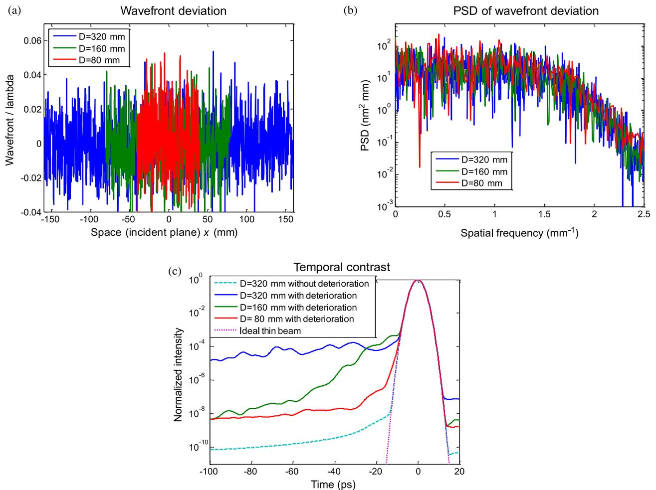
**Figure 4.** Influence of diameter on temporal contrast degradation. (a) Wavefront deviations for different diameters. (b) PSDs of wavefront deviations for different diameters. (c) Temporal contrasts for different diameters.
