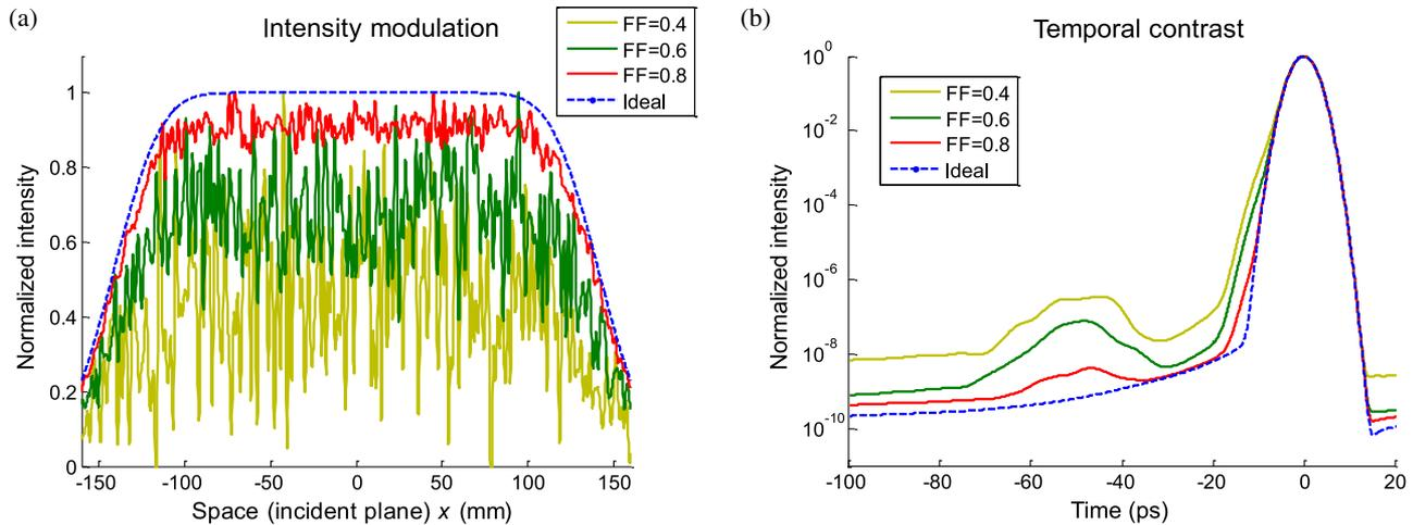
**Figure 2.** Temporal contrast degradation by intensity modulation. (a) Intensity modulation for different FFs (0.4, 0.6 and 0.8). (b) Temporal contrast for the different intensity modulations. The dashed line is the ideal situation without modulation.
