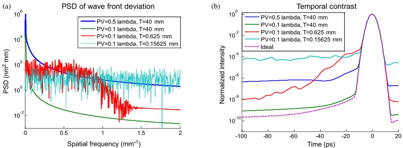
**Figure 3.** Temporal contrast degradation by wavefront deviation. (a) PSDs of wavefront deviations of different magnitudes and spatial frequencies. (b) Temporal contrasts for different wavefront deviations.
