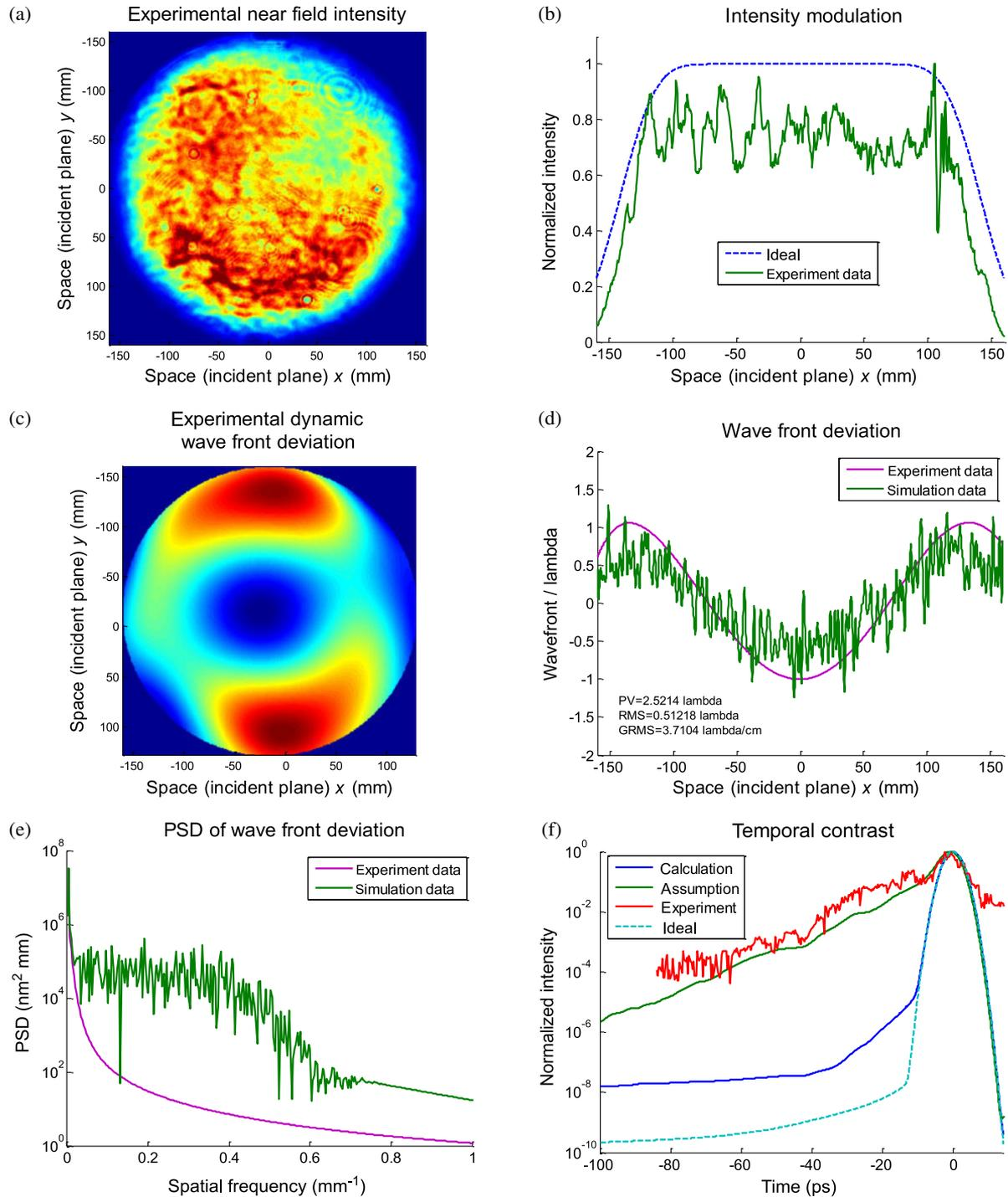
**Figure 5.** Experimental and simulated intensity modulation, wavefront deviation and temporal contrast degradation. (a) Experimental near-field intensity. (b) Intensity modulation. (c) Experimental dynamic wavefront deviation. (d) Wavefront deviation. (e) PSD of wavefront deviation. (f) Temporal contrast.
