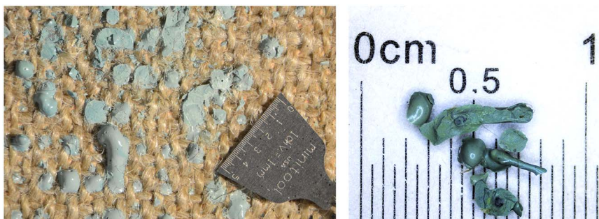
Figure 2 Sampling of the green paint P05 on the rear of the painting (→48.6 cm, ↑25.2 cm). On the left, after sample collection the respective damage can be observed. The used scale represents 5 mm. On the right, the collected sample weighed 8.5 mg. (See online version for color.)
