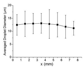
**Fig. 5.** Average diameter of pure-water droplets in the microdroplet fusion mass spectrometry as a function of the distance (x). Few noticeable differences were observed in the average size of microdroplets up to the distance of about 7 mm from the droplet fusion center. All kinetic measurements shown in Fig. 4 are performed at distances of 4 mm or less.
