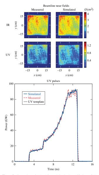
**Figure 8.** Comparison of *PSOPS* forward-simulated amplified near-field beam profiles, pulse shapes and corresponding energies with measurements for beamline 3 shot 20,678. IR: 3112 J measured, 3102 J simulated. UV: 453 J measured, 452 J simulated. Simulations used measured injected beam profile, pulse shape and energy for shot 20,678.
