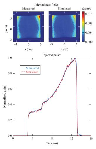
**Figure 9.** Comparison of *PSOPS* backward-simulated injected near-field beam profile, pulse shape and corresponding energy with measurements for beamline 3 shot 20,678: 79.5 mJ measured, 76.9 mJ simulated. Simulations used measured UV-beam profile, pulse shape and energy for shot 20,678.
