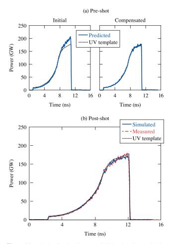
**Figure 11.** (a) Predicted and requested UV pulse shapes showing how day-to-day changes in regen performance are compensated using *PSOPS* predictions; (b) post-shot UV pulse simulation, measurement and corresponding energies (beamline 3 shot 22,254). On-target UV energy: 775 J requested, 751 J measured, 752 J simulated.
