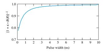
**Figure 4.** Pulse-width dependence of empirical scaling factor  $[\gamma(R)]^{-1} = [1 + K \cdot B(R)]^{-1}$  to account for finite lifetime of the terminal laser level in Nd-doped phosphate laser glass, as per Ref. [41].
