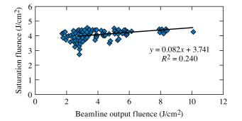
**Figure 3.** Plot of the inferred saturation fluence versus beamline output fluence from optimization fits to OMEGA EP beamline 3 data for nine-main-amplifier and seven-booster-amplifier configuration. Only shots with pulse widths and beam output energies  $\ge 2$  ns and  $\ge 2$  kJ, respectively, were used in the fit.
