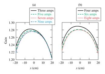
**Figure 6.** Horizontal lineouts of column-averaged, beamline 1 single-disk, small-signal gain maps for different numbers of main-amplifier disks fired. (a) Odd number of cavity amplifiers; (b) even number of cavity amplifiers.
