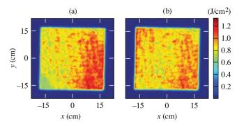
**Figure 14.** Measured beamline 3 output IR near-field beam-fluence profile (a) before moving the beam-shaping apodizer (contrast = 13.1 %, peak to mean = 1.46:1) and (b) after moving the apodizer by 0.49 mm (contrast = 9.4%, peak to mean = 1.43:1). Contrast is defined in the text. The apodizer adjustment was guided by *PSOPS* simulations.
