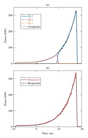
**Figure 13.** (a) Pre-shot prediction and (b) measurement of approximately 27-ns composite UV pulse formed by incoherent addition of the individual beamline pulse shapes and beam-to-beam timing (shot 31,182).
