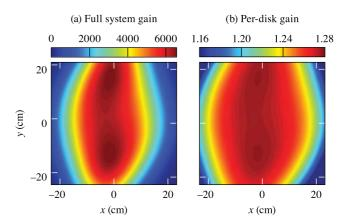
**Figure 5.** (a) Fifteenth-order Legendre fit to the measured total small-signal gain for beamline 1, nine-main-amplifier configuration and (b) its *N*th root (geometric mean) for the nine-disk, four-pass cavity where N = 36. The single-disk small-signal gain shown in (b) is used in the *PSOPS* model when nine main amplifiers are configured for beamline 1.
