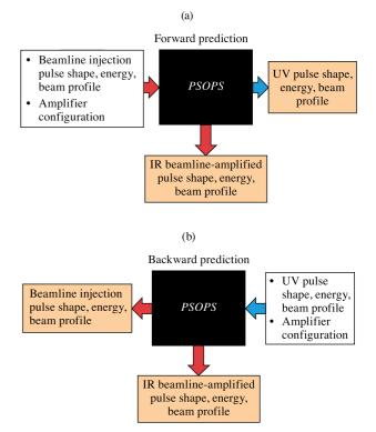
**Figure 2.** Beamline pulse shape, energy and near-field beam profile are predicted in real time by *PSOPS* in forward and backward directions. (a) Forward prediction – UV beamline output is predicted using inputs to the amplifier chain and a specified amplifier configuration. (b) Backward prediction – IR stage energies, pulse shapes and near-field profiles are predicted using specified UV inputs and amplifier configuration.
