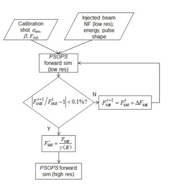
**Figure 7.** Flowchart illustrating the quasi-Newton method used for *PSOPS* forward predictions with a low-resolution grid. On the first iteration, the spatially-averaged output beam fluence  $F_{out}$  is compared to  $F_{out}$  from the calibration shot. The saturation fluence  $F_{sat}$  is then scaled per the previously measured  $F_{sat}$  vs.  $F_{out}$  slope. Pulse-width correction to  $F_{sat}$  is applied before the final (high resolution) simulation.
