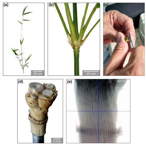
Figure 7: Sample preparation of bamboo (*B. tuldoides*) for X-ray microtomography: (a) top portion of the stem; (b) nodal region of the apical stem of the specimen, consisted of a primary axis generating lateral sheaths and buds; (c) cross-sectioning of the sample; (d) sectioned sample; (e)  $\mu$ CT projection.
