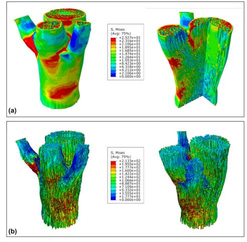
Figure 6: The von Mises stress results at the compressive failure of the μCT-based FEA of the nodal region of bamboo: (a) parenchyma elements set only, and internal view cut; (b) sclerenchyma elements set only. Mesh elements contours were hidden to improve the visualization of the colored regions.
