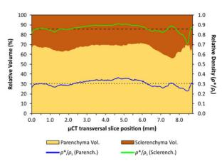
**Figure 4:** Relative volume (%) and relative density ( $\rho^*/\rho_s$ ) of parenchyma and sclerenchyma related to each transversal slice position of the  $\mu$ CT-segmented nodal bamboo. Dotted and dashed lines represent the average values of  $\rho^*/\rho_s$  for the parenchyma and sclerenchyma, respectively.
