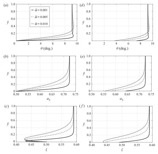
Figure 2. The influence of the diffusion coefficient,  $\bar{\alpha}$ , on the orientational angle, nematic order and ordering fields for  $\bar{\nu} = 0$  and  $\bar{\nu} = 0.05$ : (a)  $\bar{\nu} = 0$ , (b)  $\bar{\nu} = 0$ , (c)  $\bar{\nu} = 0$ , (d)  $\bar{\nu} = 0.05$ , (e)  $\bar{\nu} = 0.05$  and (f)  $\bar{\nu} = 0.05$ .
