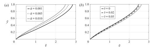
Figure 4. The influence of the diffusion coefficient,  $\bar{\alpha}$ , and orientational boundary jump coefficients,  $\bar{\nu}$ , on the velocity profile: (a)  $\bar{\nu} = 0$  and (b)  $\bar{\alpha} = 0.01$ .
