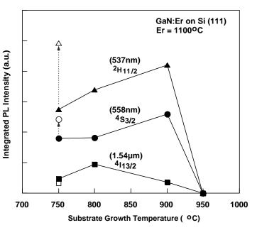
**Figure 2:** Integrated PL intensity of Er emission from samples grown on Si as a function of growth temperature. The open symbols represent a different buffer layer.
