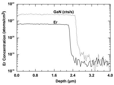
Figure 5: SIMS depth profile of Er concentration from film grown on Si. Er cell =  $1100^{\circ}$ C.
