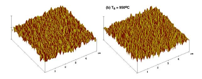
**Figure 3:** AFM images of the GaN:Er films on Si (111). Growth temperature was (a) 750°C and (b) 950°C. Er cell temperature was 1100°C.
