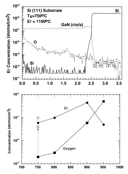
Figure 7: Concentration of Er and O as a function of growth temperature. The open symbols represent a different buffer layer. Er cell =  $1100^{\circ}$ C.
