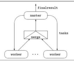
Fig. 10. Master-worker process topology.
