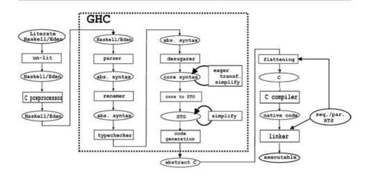
Fig. 17. Overview of the GHC with extensions for Eden.
