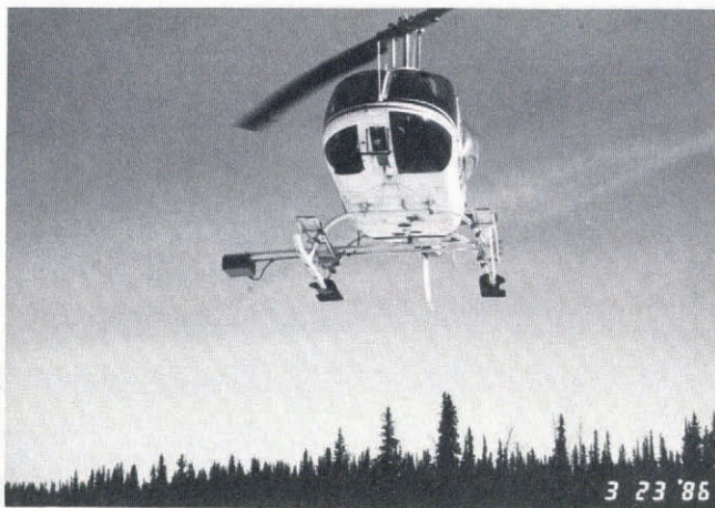
Fig. 1. Bell 206B Jet Ranger with 3102 antenna unit mounted to the side.
