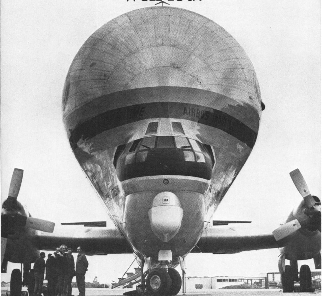
This bulbous leviathan is the Super Guppy. A derivative of the Boeing Stratocruiser, its 35,000 cu. ft. cargo hold is the largest of any aircraft in the world. The Super Guppy flies regularly between Manchester Airport and the Airbus Industrie works at Toulouse, transporting sets of wings made at Hawker.
