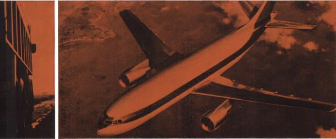
The wings of the A300B European Airbus were designed and fabricated by Hawker Siddeley Aviation. In their constructions H.D.A. aluminium alloy precision forgings were used.
