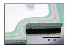
Figure 1. Alternating strip opal heterostructures obtained inside capillary cells with a special shape. Reprinted in part with permission from Chemistry of Materials 17(15)(2005) p. 3809; DOI: 10.1021/cm051114i. © 2005 American Chemical Society.
