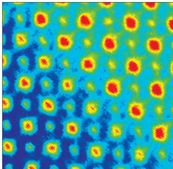
High-angle annular dark-field scanning transmission electron microscope image of the transition from LSMO to PZT (bottom left to top right). Localized polarization occurs at the LSMO/PZT interface due to the ferroelectric properties of the PZT layer. Credit: James Rondinelli.
