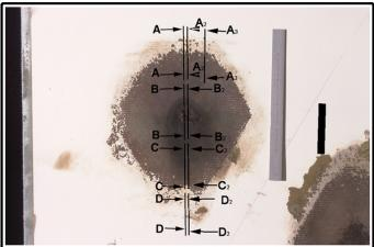
Figure 2: A section map of a lab induced lightning strike on a honeycomb carbon fiber composite structure that contained an expanded wire aluminum mat.
