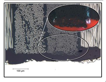
Figure 3. A carbon fiber composite showing a hot spot due to intraply arcing. It has been backfilled with rhodamine B laser dyed epoxy. This shows the voided zone adjacent and around the center of the hot spot. Polarized light illumination.
