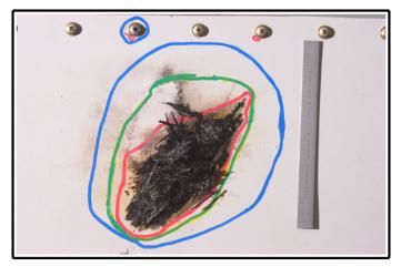
Figure 1: A lab induced lightning strike on a carbon fiber composite.
