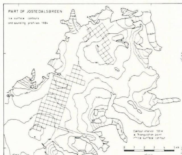
Fig.2. Ice surface contours and sounding profiles.
