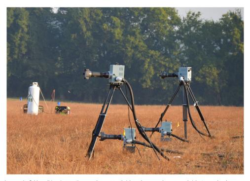
Figure 1. Air samplers shown under field conditions in 2017. Two samplers at 0.3 m height and two samplers at 1.3 m height. Image also shows propane-powered generators used to provide electrical power to operate samplers. Surface treatment shown is dry wheat stubble.
