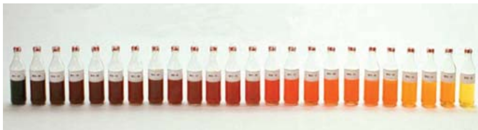
Oil composition can vary significantly within the reservoir. All of these samples were extracted from a single column. Image courtesy of Hani Elshahawi, Shell International E&P.
