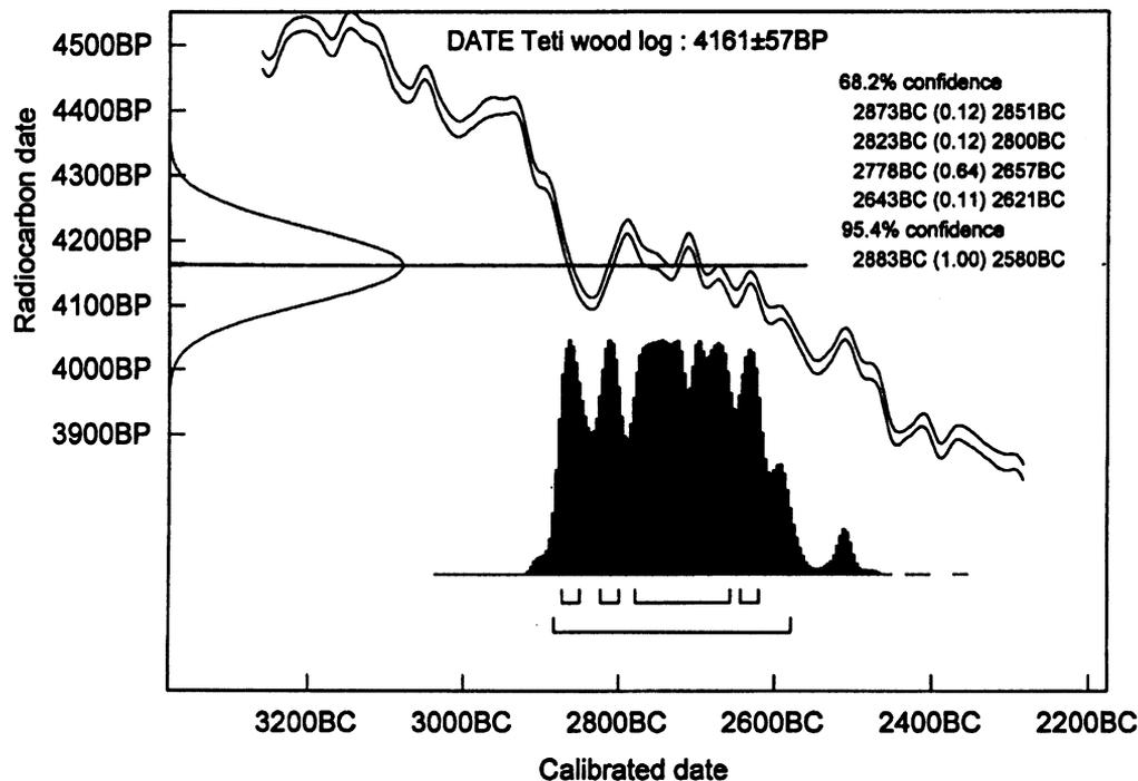
Fig. 1.  $^{14}\text{C}$  date intersecting a flat portion of the calibration curve, producing 5 intersections and a 252-yr wide probability distribution with a  $1-\sigma$  confidence level
