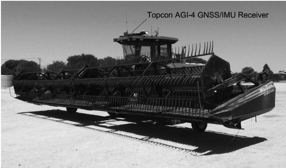
Figure 2. MacDon 9300 Self-Propelled Windrower with Topcon AGI-4 GNSS/IMU Receiver.
