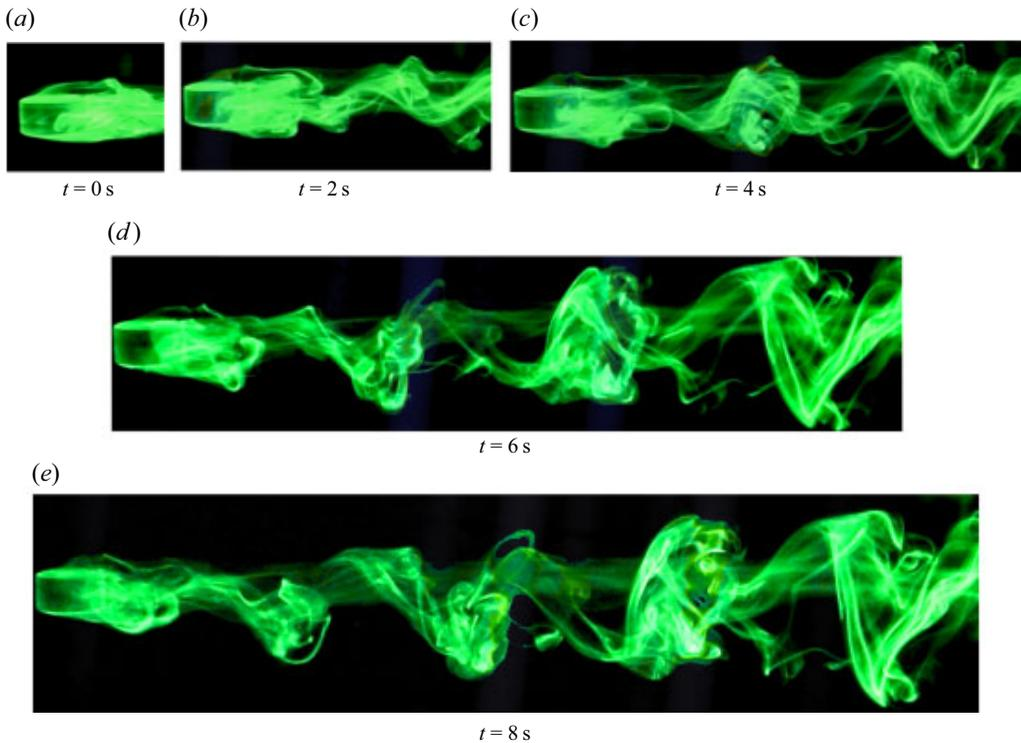
Figure 20. Plan view of experimental flow visualisation using UV-induced fluorescent dye technique. Temporal evolution of the wake of a freely rolling cylinder D19.7-A0.5 at  $\overline{Re} = 558(\pm 9)$ . The images depict the evolution of the wake from  $t = 0$  s ( $t^* = 0$ ) to  $t = 8$  s ( $t^* = 12.1$ ). Cylinder rolling from right to left. The video recordings are provided as supplementary movie 4 available at <https://doi.org/10.1017/jfm.2024.833>.
