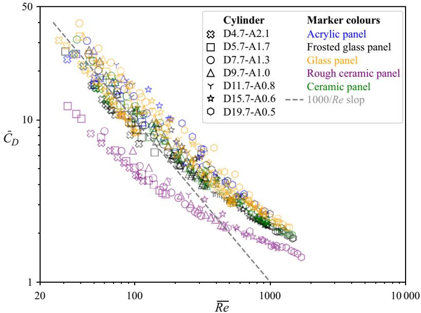
Figure 4. Variation of  $\bar{C}_D$  with  $\bar{Re}$  for the five types of panels,  $\bar{Re} = 20\text{--}1800$  range in log–log scale. The cylinder span was fixed at 10.1 mm which results in varied AR ranging from 0.51–2.15.
