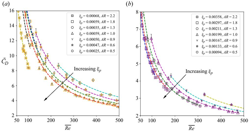
Figure 6. Variation of  $\bar{C}_D$  with  $\bar{Re}$  for cylinders of different diameter rolling on the (a) glass panel and (b) rough ceramic panel. Least-squares lines of the form  $a + b/Re$  have been fitted through data that correspond to the individual diameters of the cylinders used. The  $R^2$  values are approximately 0.9. Error bar indicate bias error only.
