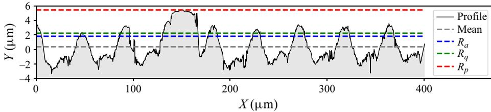
Figure 2. Visual representation of the three roughness statistics on a sample cylinder profile.
