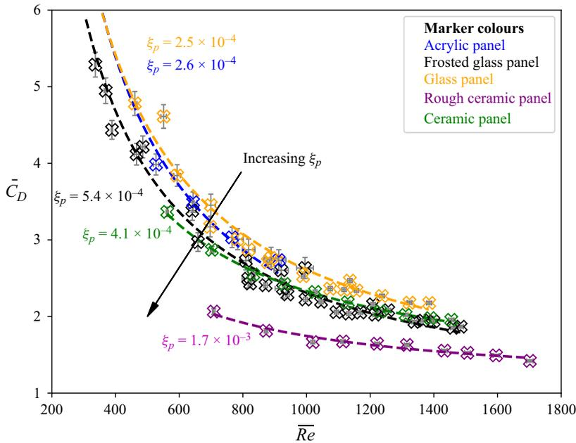
Figure 5. Variation of  $\bar{C}_D$  against  $\bar{Re}$  for a cylinder with a fixed diameter and aspect ratio, D19.7-A0.5, while varying the panel surface roughness. Least-squares lines of the form  $a + b/Re$  have been fitted through data that correspond to individual panels. The coefficient of determination  $R^2$  values are approximately 0.9.
