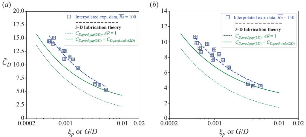
Figure 10. Variation of  $\bar{C}_D$  with  $\xi_p$  for  $AR \approx 1$  at (a)  $\overline{Re} = 100$  and (b)  $\overline{Re} = 150$ . A line of best fit of the form  $a + b/\sqrt{\xi}$  is used to show the general trend with  $R^2$  approximately 0.9.
