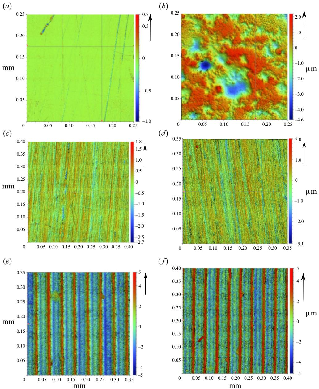
Figure 3. Surface roughness profiles obtained using the optical profilometer, under 50 $\times$  magnification: (a) acrylic panel; (b) ceramic panel; (c) D4.7-A2.2 cylinder; (d) D7.7-A1.3 cylinder; (e) D11.7-A0.9 cylinder; (f) D19.7-A0.5 cylinder. The arrow at the top right corner of each panel image indicates the approximate down-slope direction, whereas for cylinder images, the arrow shows the direction of rolling of each cylinder, with respect to the directional surface textures.
