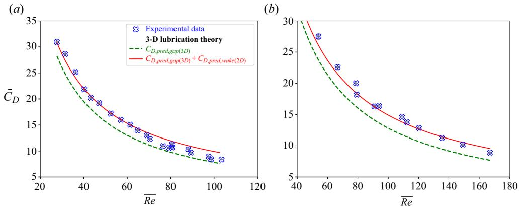
Figure 7. Comparison of  $\bar{C}_D$  vs  $\bar{Re}$  of two cylinders rolling on a glass panel against analytical prediction (2.8). The total drag when two-dimensional  $C_{D,pred,wake}$  predictions from (2.7) is added to (2.8) is also indicated in the figure. Physical parameters are (a)  $\xi_{p,1\sigma} = 0.00096$  and  $AR = 2.16$  and (b)  $\xi_p = 0.00035$  and  $AR = 1.31$ .
