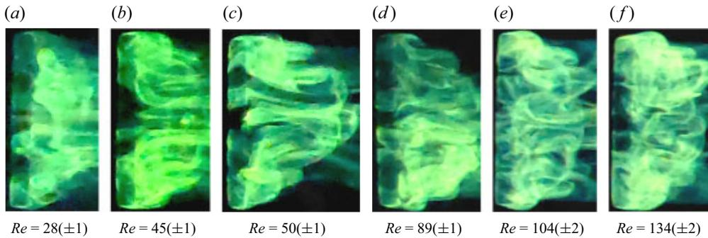
Figure 15. Plan view of experimental flow visualisation using UV-induced fluorescent dye technique. Comparison of the near wake of a freely rolling cylinder D4.7-A10.7 with  $\overline{Re}$  ranging from 28–134, for a constant  $D$  (4.69 mm). Cylinder rolling from right to left. The video recordings are provided as supplementary movie 2 available at <https://doi.org/10.1017/jfm.2024.833>.
