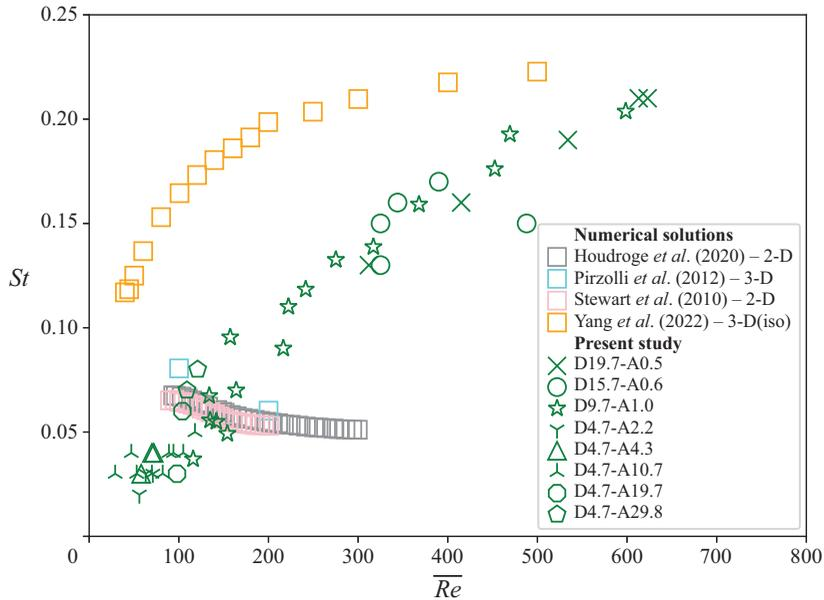
Figure 21. Comparison of  $St$  vs  $\overline{Re}$  variation for a freely rolling cylinder with varied aspect ratios ( $\approx 0.5$ – $30$ ) and diameters. For experimental data, Stewart *et al.* (2010a) and Yang *et al.* (2023) the  $St$  of vortex shedding is shown. For Houdroge *et al.* (2020) and Pirozzoli *et al.* (2012) the  $St$  of oscillations is indicated. Numerical predictions from previous literature have also been plotted for comparison.
