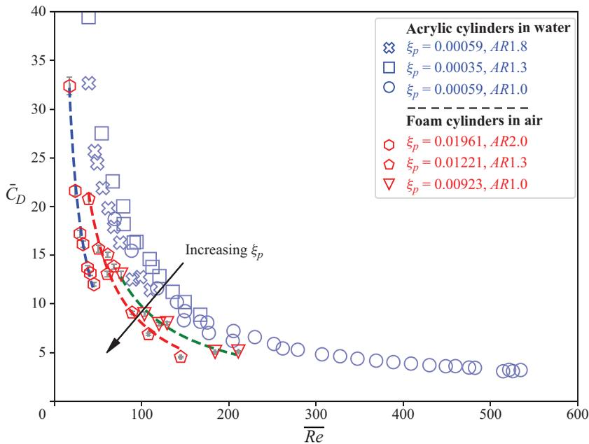
Figure 9. Variation of  $\bar{C}_D$  with  $\bar{Re}$  for foam cylinders rolling in the air on the glass panel. The cylinder span was fixed for all measurements ( $L = 10.1$  mm) while the aspect ratio varied. The results of acrylic cylinders in water are also plotted for comparison.
