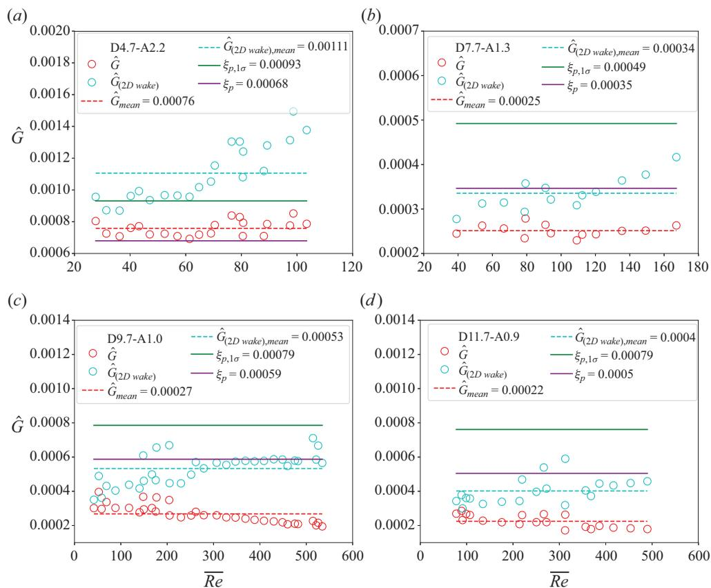
Figure 11. Non-dimensional effective gap ( $\hat{G} = G_{eff}/D$ ) vs  $\overline{Re}$  for four cylinders rolling on a smooth glass panel: (a) D4.7-A2.2 cylinder; (b) D7.7-A1.3 cylinder; (c) D9.7-A1.0 cylinder; (d) D11.7-A0.9 cylinder. Cylinder span  $L = 10.1$  mm for all diameters. The measured roughness parameters of the cylinders are plotted in the figure.
