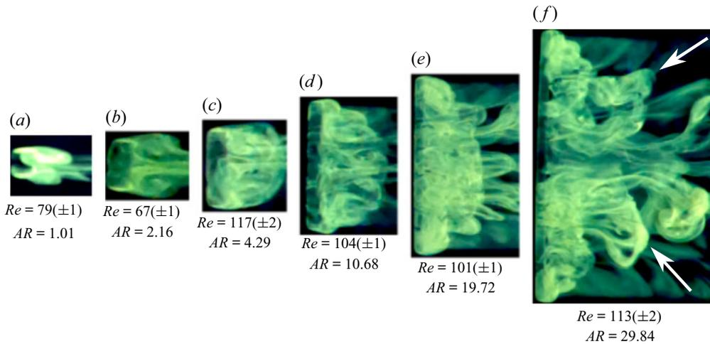
Figure 16. Plan view of experimental flow visualisation using UV-induced fluorescent dye technique. Comparison of the near wake of a freely rolling cylinder, for different  $AR$  ranging from 1.01 to 29.84, for a constant  $D$  (4.7 mm) and  $\theta = 14^\circ$ . Cylinder rolling from right to left. White arrows indicate the shedding of a pair of vortices per shedding cycle. The video recordings are provided as supplementary movie 3 available at <https://doi.org/10.1017/jfm.2024.833>.
