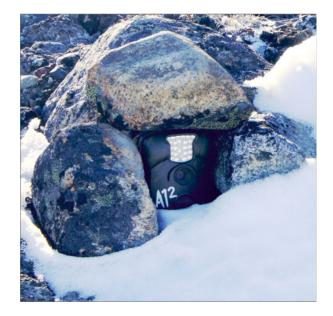
Fig. 2. Example of a trail camera installation at the lake shore.
