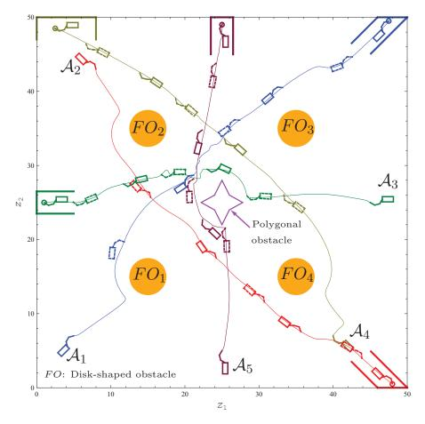
Fig. 9. Scenario 2. The resulting trajectories of the 3DNMs with angle-gain parameters,  $\rho_{i0} = 1$ ,  $\rho_{ik} = 1$ , k = 1, 2, 3 and convergence parameters  $\delta_{ij} = 550, j = 1, \dots, 4$ .
