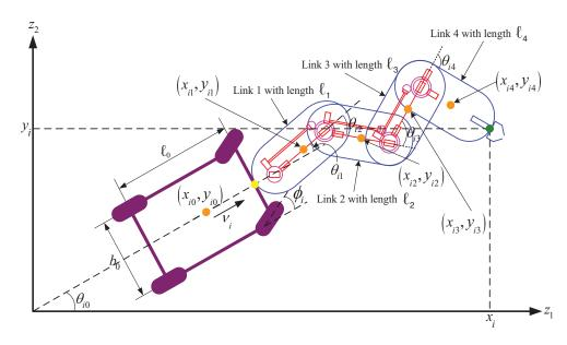
Fig. 1. Illustration of the ith 4DNM in the inertial frame  $\mathcal{F}$ . The schematics of the 4-link nonholonomic manipulator is adopted from.<sup>29</sup>
