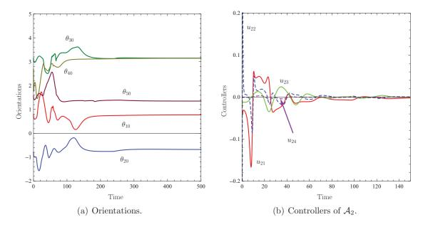
Fig. 10. Scenario 2. (a) shows the evolution of the orientations of the wheeled platforms of the 3DNMs while (b) depicts the progression of the acceleration controllers of  $A_2$ . (a) Orientations. (b) Controllers of  $A_2$ .
