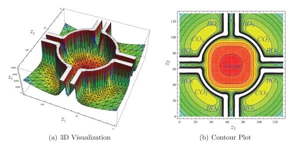
Fig. 6. The total potentials (corresponds to the  $z_3$ -axis) for target attraction and avoidance of multiple rod-shaped and curve-shaped obstacles by the wheeled platform of a 3DNM with the target fixed at  $(p_{11}, p_{12}) = (65, 65)$ . Also,  $v_1 = 2$ ,  $\omega_{10} = \omega_{11} = \omega_{12} = \pi/360$ ,  $\theta_{10} = 0$ ,  $\theta_{11} = \pi/3$ ,  $\theta_{12} = -\pi/3$ , and  $\theta_{13} = -\pi/4$ . (a) 3D visualization. (b) Contour plot.
