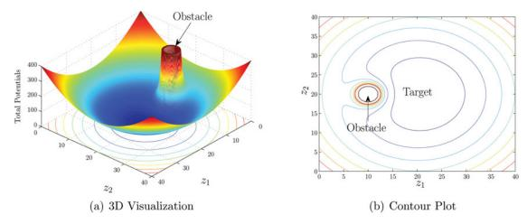
Fig. 3. The total potentials generated by Eq. (4). The target is located at  $(p_1, p_2) = (20, 20)$  with radius  $r_T = r_P = 1$  and the obstacle is fixed at  $(o_1, o_2) = (10, 20)$  with a radius of  $r_Q = 2$ . The value of the tuning parameter is chosen as  $\alpha = 10$ . (a) 3D Visualization. (b) Contour plot.
