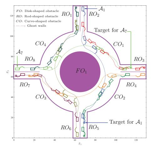
Fig. 7. Scenario 1. The resulting trajectories of the 3DNMs with dimensions  $\ell_0 = 1.5$ ,  $b_0 = 0.7$  and  $\ell_1 = \ell_2 = \ell_3 = 0.7$ . Also,  $\rho_{i0} = 1$ ,  $\rho_{ik} = 1$  (k = 1, 2, 3),  $\delta_{ij} = 200$ ,  $j = 1, \ldots, 4$ , the initial velocities are  $v_i(0) = 3$ ,  $\omega_{i0}(0) = 0.2$ , and  $\omega_{i1}(0) = \omega_{i2}(0) = 0.05$ , for  $i = 1, \ldots, 8$ .
