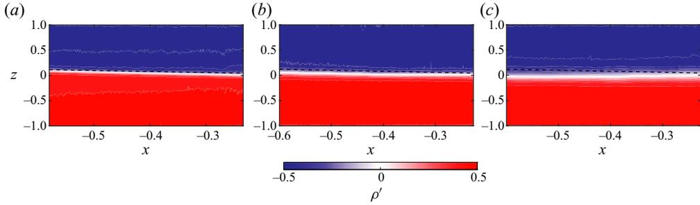
Figure 5. Time-averaged density field in the  $(x, z)$  plane at  $y = 0$  for three experiments in the mSID set-up. (a) Experiment within the L regime ( $\theta = 2^\circ$ ,  $Re_g = 398$ ). (b) Experiment within the H regime ( $\theta = 2^\circ$ ,  $Re_g = 1059$ ). (c) Experiment within the I regime ( $\theta = 2^\circ$ ,  $Re_g = 1455$ ). The black dashed line represents the line  $z = Sx$  with  $S = -0.20$  as given by (3.37).
