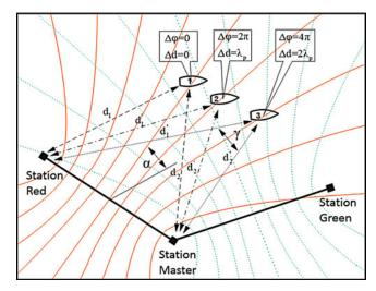
Figure 4. Principle of operation of DNS (Urbański and Posiła, 1966).
