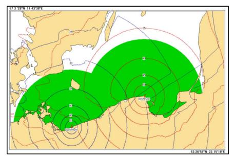
Figure 8. Coverage of Polish DGPS reference stations in 2014 (Śniegocki et al., 2014).
