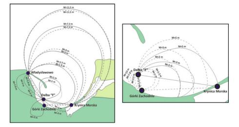
Figure 6. Accuracy zones for two variants of pairs of stations for AD-2 system (Winogradow, 1978).
