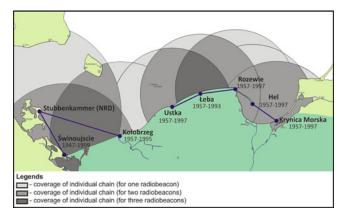
Figure 3. Coverage of individual chains (Hydrographic Office of the Polish Navy, 1971; Łysejko, 2012).
