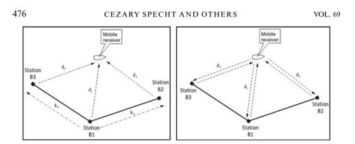
Figure 7. Principle of operation of the SYLEDIS system: in a passive (left) and in an active mode (right) (Sercel S. A., 1981).
