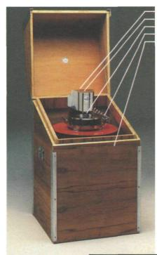
Two Way Air Control Valve Clamp Dust Cover Clamp Mounting Plate Flexible Air Line Laminated Timber Noise Reduction Cabinet
