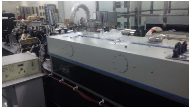
Figure 1. Multifunctional high-performance Nd:glass system based on a four-pass amplifier.
