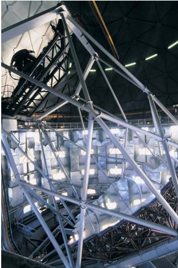
Figure 2. The SALT telescope, with the primary mirror array at the bottom right and the tracker and prime focus payload to the left, with the white dome shutter behind.
