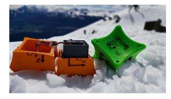
**Figure 2.** The figure displays two generation II AvaNodes employed in the experiments, namely AvaNode C10 (orange) and AvaNode C07 (green). AvaNode C10 has a density of  $\rho$  = 415 kgm $^{-3}$ , while C07 represents a density variation with a density of  $\rho$  = 688 kgm $^{-3}$ . It is important to note that the density is solely determined by the housing of the AvaNode, while the internal hardware remains consistent for both devices.
