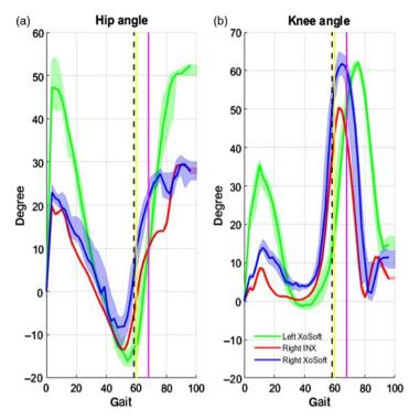
Fig. 8. Comparison of hip (a) and knee (b) joint angles of the user's left leg (healthy side). The right leg angles are displayed under the condition of wearing XoSoft and *INX*. The vertical lines represent the instant when toe off occurs for the three trends: left XoSoft (pink), right XoSoft (yellow), and right *INX* (black).
