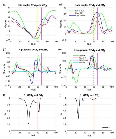
Fig. 13. Comparison of hip (a)–(c) and knee (d)–(f) joint angle, power, and assistance for right and left legs with XoSoft and *INX* under the unique control condition  $QPA_B$  and  $EB_A$ . The vertical lines represent the instant when toe off occurs.
