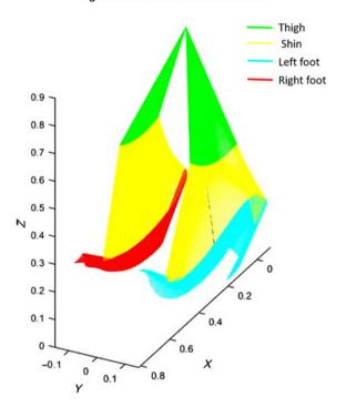
Fig. 12. Direct kinematics of lower limbs during gait.
