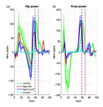
Fig. 10. Comparison of hip (a) and knee (b) joint power of left leg *INX*, right leg with XoSoft, *INX*, and the power generated by the actuator under all the control conditions (PA,  $QPA_A$ , and  $QPA_B$ ) and different *EBs*. The vertical lines represent the instant when toe off occurs for left and right gait: left (pink), right (black).
