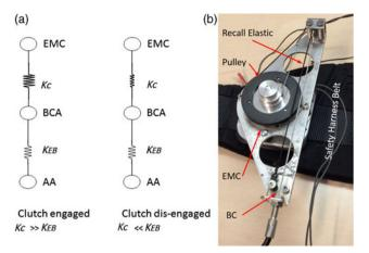
Fig. 3. (a) Mechanical schematic of the actuation unit. (b) Physical representation of the EMC and recall elastic.
