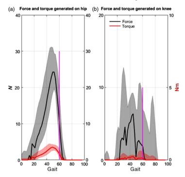
Fig. 9. Comparison of hip (a) and knee (b) joint force and torque generated on the right leg under the conditions PA,  $QPA_A$ , and  $QPA_B$ . The vertical pink line represents the instant when toe off occurs for the right leg.
