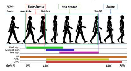
Fig. 5. Schematic of the insole sensor output, FSM, and control strategies for the right leg.
