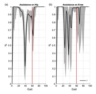
Fig. 11. Comparison of hip (a) and knee (b) assistance for the right leg with XoSoft under all the control conditions (PA,  $QPA_A$ , and  $QPA_B$ ) and different *EBs*. The vertical lines represent the instant when toe off occurs for right gait.
