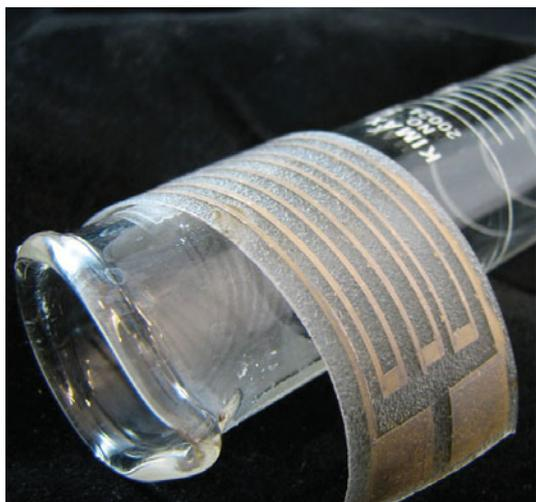
Reactive silver ink is airbrushed onto a thin, stretchy plastic film to make a flexible silver electrode. Photo by S. Brett Walker
