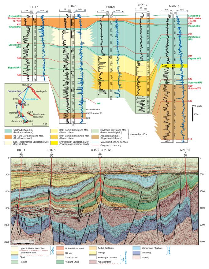
Fig. 8. Correlation panel exhibits the marked facies change from lower coastal plain deposits in BRT-1 through into open marine, shelf conditions, 20km north in MKP-16. The Tertiary Laramide event inverted the basin centre whilst subsidence continued in the south resulting in a southerly tilt to the basin.
