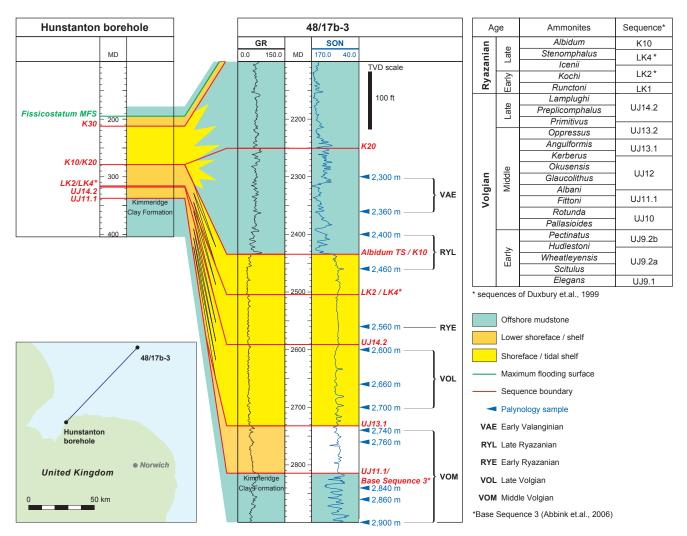
Fig. 5. Jurassic/Cretaceous boundary successions of the Hunstanton borehole and Sole Pit Basin. The UJ11.1 mid Volgian Cimmerian Unconformity marks the final separation of a marine connection between the Wealden Basin and the southern North Sea Basins.
