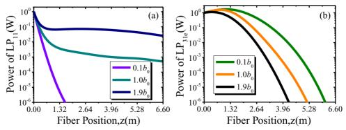
Figure 11. Power evolution of (a)  $LP_{11}$  mode and (b)  $LP_{31e}$  mode in the T-SCF under a bending radius of 32 cm.
