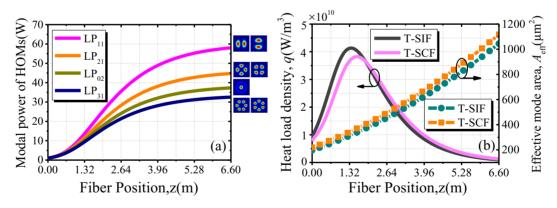
Figure 10. (a) Modal power evolution of four HOMs in linear T-SIF and (b) comparison of heat load density and effective mode area of LP<sub>01</sub> between linear T-SCF and T-SIF.
