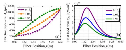
Figure 9. (a) Effective mode area of  $LP_{01}$  and (b) heat load density evolution along T-SCF.
