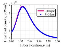
Figure 12. Comparison of heat load density between straight T-SCF and bent T-SCF of R = 32 cm.
