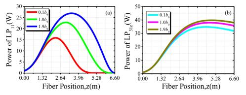
Figure 14. Modal power evolution of (a)  $LP_{11}$  mode and (b)  $LP_{31e}$  mode for concave, linear, and convex T-SCF under the large-to-small amplification scheme.
