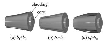
**Figure 2.** Three major tapered categories: (a) concave tapered fiber, (b) linear tapered fiber, and (c) convex tapered fiber.
