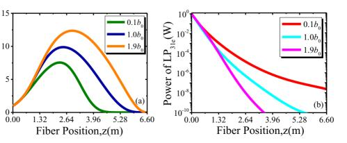
Figure 16. Power of (a) LP<sub>11</sub> and (b) LP<sub>31e</sub> of the T-SCF under a bending radius of 32 cm.
