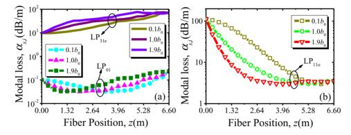
Figure 5. Comparison of modal loss of T-SCF with a bending radius of 32 cm: (a) mode losses of LP<sub>01</sub> and LP<sub>31e</sub>; (b) mode loss of LP<sub>110</sub>.
