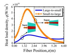
Figure 15. Comparison of heat load density between the two amplification schemes.
