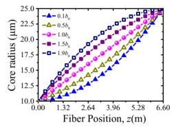
**Figure 3.** Effects of different parabolic shape factors on the core radius profile (from the small end to the large end).
