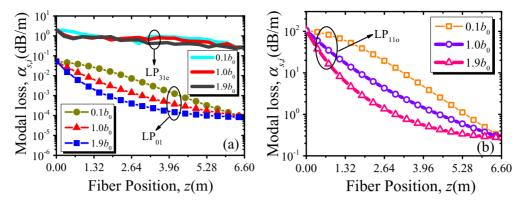
Figure 4. Comparison of modal loss of straight T-SCF from the small end to the large end: (a) mode losses of LP<sub>01</sub> and LP<sub>31e</sub>; (b) mode loss of LP<sub>11o</sub>.
