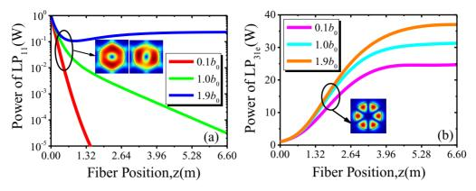
Figure 8. Modal power evolution of (a) LP<sub>11</sub> mode and (b) LP<sub>31e</sub> mode for concave, linear, and convex T-SCF based on the small-to-large amplification scheme.
