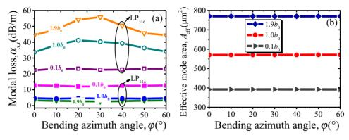
Figure 6. (a) Modal loss and (b) effective mode area of LP<sub>01</sub> for T-SCF under various bending azimuth angles, R = 32 cm, and z = 3.3 m.
