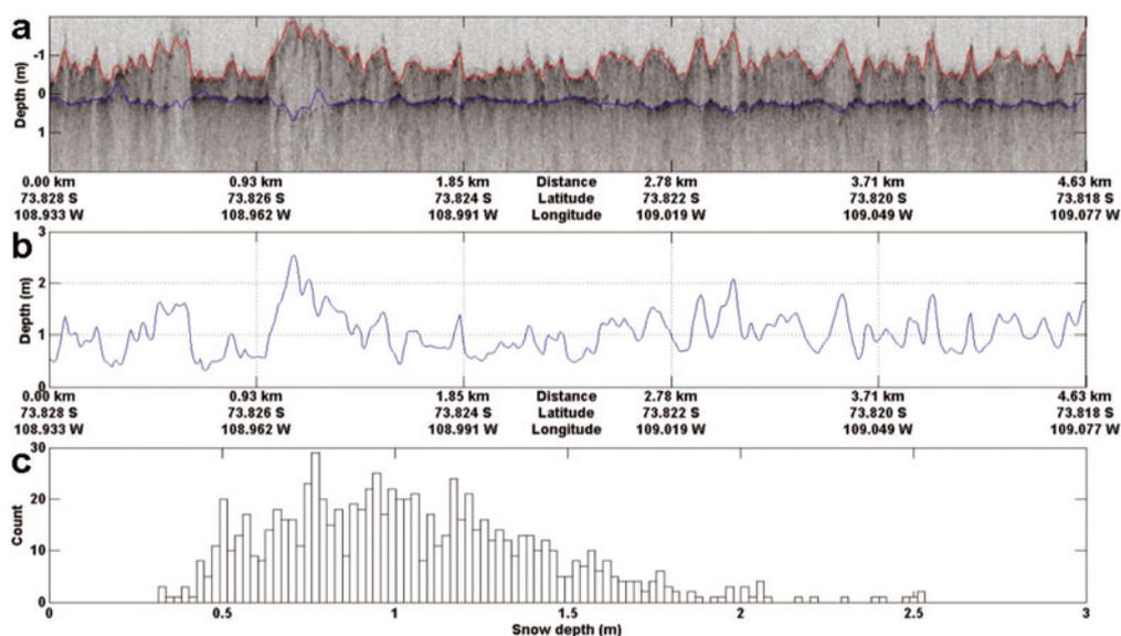
**Fig. 9.** Standard output from the interface tracker. (a) Extracted air/snow and snow/ice interfaces from the echogram presented in Figure 8. (b) Snow depth vs. along-track position. (c) Histogram of snow thickness derived assuming a constant snow density of  $0.3 \text{ g cm}^{-3}$ . Mean snow thickness for the segment was 93 cm.
