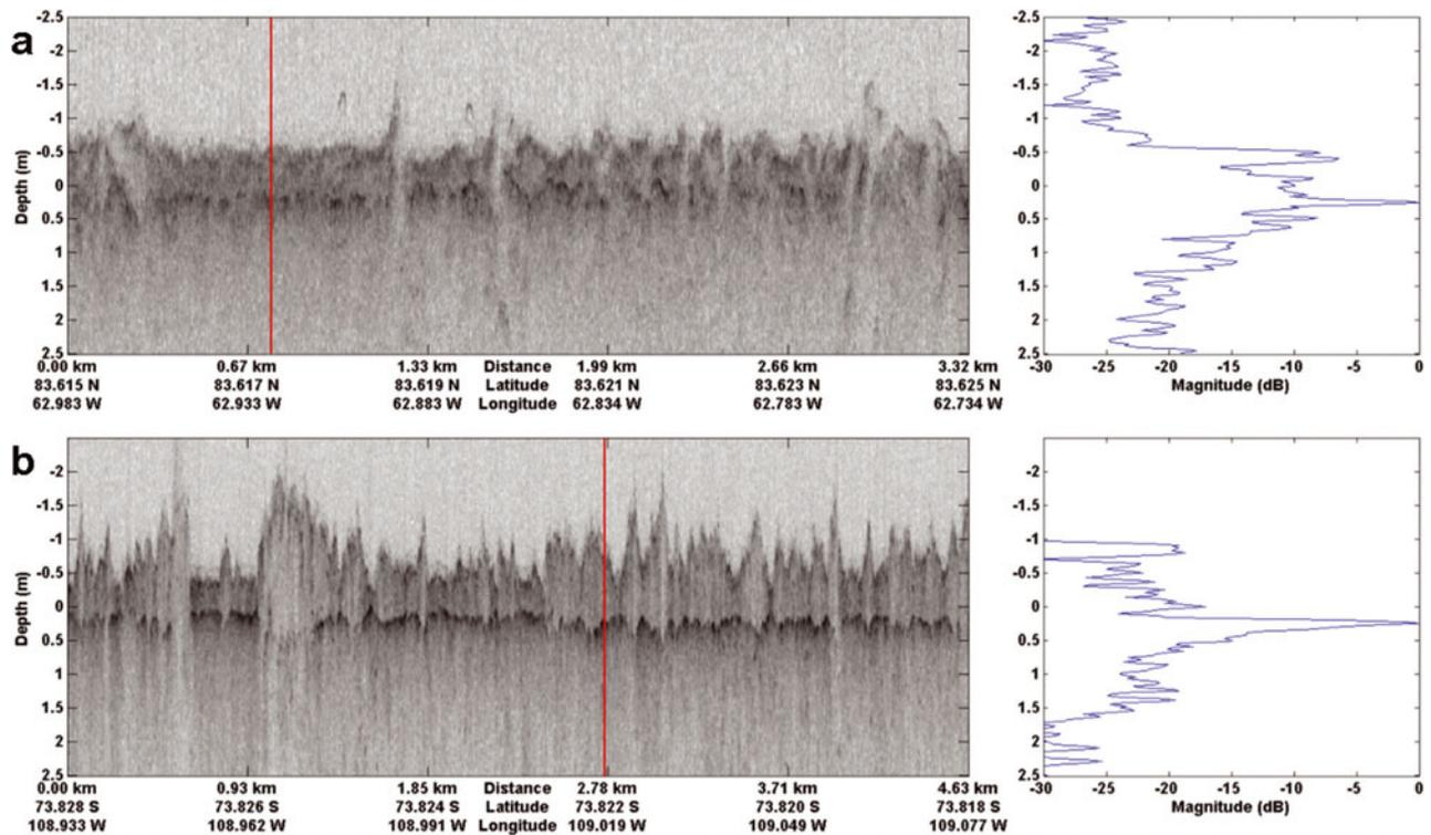
**Fig. 10.** Comparison between radar returns from the snow/ice interface for the Arctic (a) and Antarctic (b) sea ice. The second interface shown in echogram of (b) is believed to be a snow/slush interface due to the increase in the relative amplitude offset between the two interfaces.
