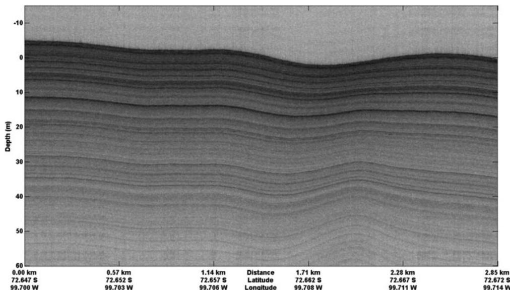
**Fig. 7.** Snow Radar results from the 9 November 2009 Pine Island Glacier flight showing the improvement in SNR from the coherent noise removal method applied to the data in Figure 6a. A constant snow density of  $0.3 \text{ g cm}^{-3}$  was assumed. Firn snow density increases with depth, so the depth axes overestimate the depth for deeper targets.
