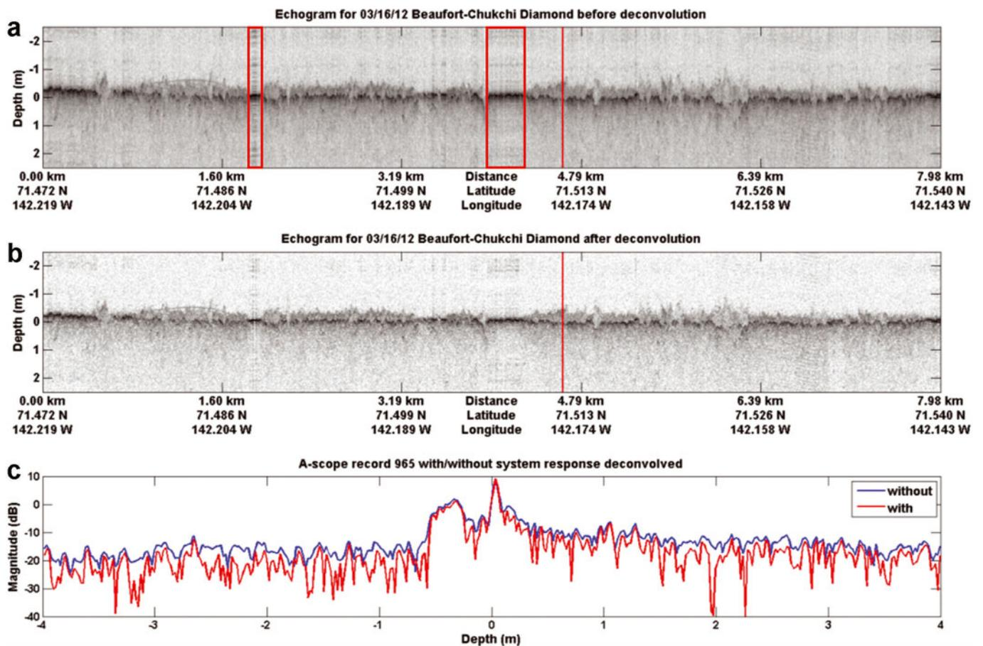
**Fig. 11.** Snow Radar results from the 16 March 2012 Beaufort–Chukchi flight in the Arctic. (a) Echogram for eight data files (Nos. 163–170) without compensating for the system response. (b) The same echogram with the system response deconvolved. (c) Comparison of the A-scopes at the location marked with the line. Average system response was derived from the A-scopes lying within the boxes outlined in (a).
