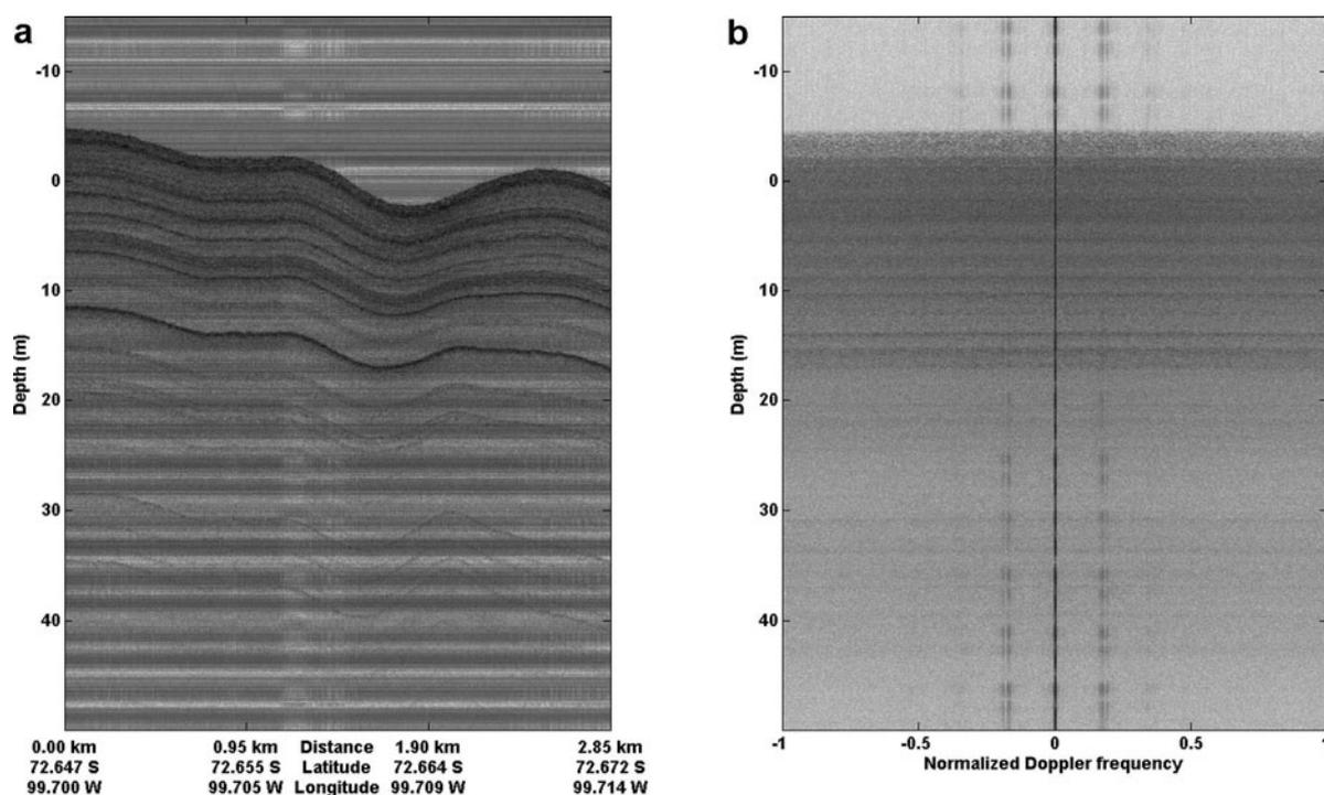
**Fig. 6.** (a) Radar echogram from 9 November 2009 Pine Island Glacier (Antarctica) flight which demonstrates the coherent noise present in the collected data which restricts useful data to the top 10 m. (b) The same data are displayed in the range-Doppler domain, and the strong zero-Doppler component can be clearly seen.
