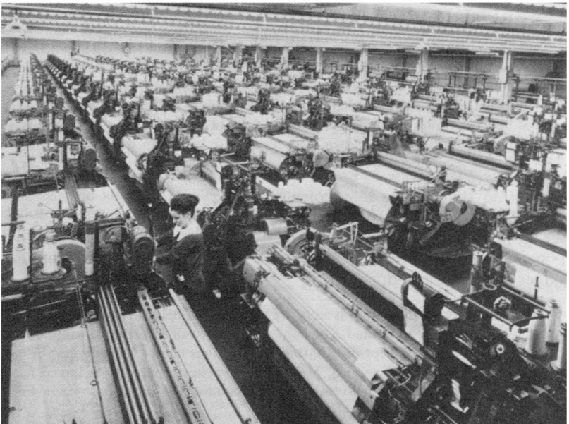
A Weaving Shed Built in 1966 with Automatic Looms.
