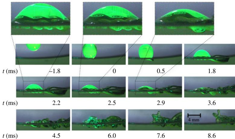
FIGURE 4. (Colour online) Time evolution of the impact of a droplet with viscosity  $5 \text{ mPa s}$  at a normal speed of  $1.3 \text{ m s}^{-1}$  onto a pool of the same liquid moving from left to right at  $3.3 \text{ m s}^{-1}$ . Laser and colour high-speed imaging were combined to observe the mixing process; the impacting droplet contained  $0.02\%$  fluorescein. See also supplementary movie 4.
