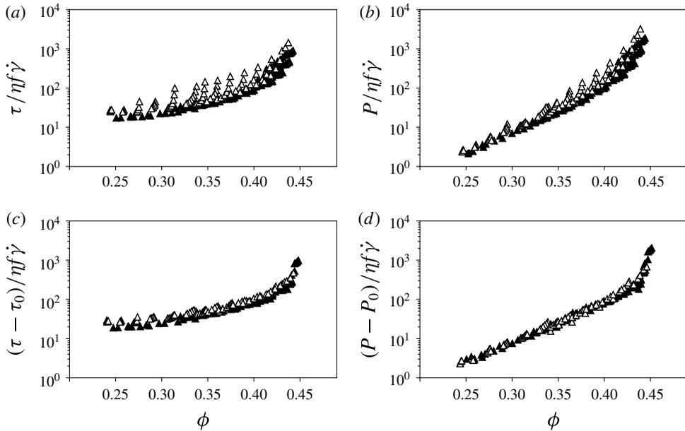
FIGURE 2. Apparent relative (a) shear ( $\tau/\eta_f\dot{\gamma}$ ) and (b) normal ( $P/\eta_f\dot{\gamma}$ ) viscosities as well as relative (c) shear ( $(\tau - \tau_0)/\eta_f\dot{\gamma}$ ) and (d) normal ( $(P - P_0)/\eta_f\dot{\gamma}$ ) viscosities (after subtraction of the yield stresses) versus volume fraction,  $\phi$ , for the fibres of batch (II) in pressure-imposed ( $\blacktriangle$ ) and volume-imposed ( $\triangle$ ) configurations.
