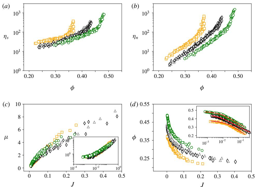
FIGURE 4. Rheological data: (a)  $\eta_s = (\tau - \tau_0)/\eta_f \dot{\gamma}$  and (b)  $\eta_n = (P - P_0)/\eta_f \dot{\gamma}$  versus  $\phi$  as well as (c)  $\mu = \eta_s/\eta_n$  and (d)  $\phi$  versus  $J = \eta_f \dot{\gamma}/(P - P_0)$ , for fibre batches (I), (II), (III) and (IV) as represented by the symbols  $\square$ ,  $\Delta$ ,  $\diamond$  and  $\circ$ , respectively (see table 1). The insets of graphs (c,d) are log-log and semilogarithmic plots.
