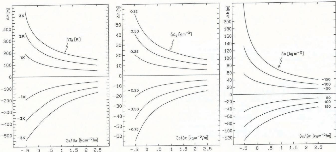
Fig. 4. Altitudinal shift of the equilibrium line versus the gradient of annual accumulation for perturbations of air temperature  $\delta T_a$  (left), absolute humidity  $\delta \rho_v$  (center) and annual accumulation  $\delta c$  (right).
