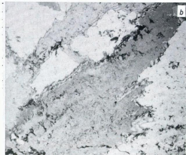
Fig. 8. Photomicrographs of horizontal sections illustrate the sub-structure of (a) congelation ice in core RS-24, 0.86 m, (b) platelet ice in core RS-27, 2.10 m and (c) congelation ice located in the interstices between platelets in core RS-29, 2.08 m. Scale divisions are at 1 mm intervals.
