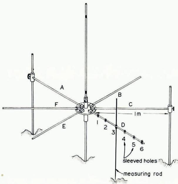
Fig. 6. *The star ablatometer.*
