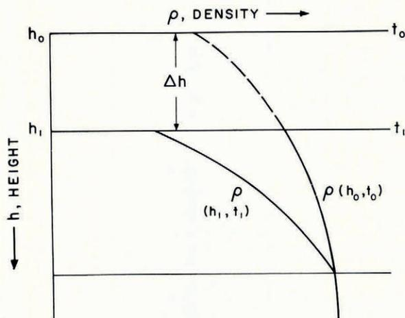
Fig. 7. Two successive ideal depth–density curves on a melting glacier (after LaChapelle, 1959).
