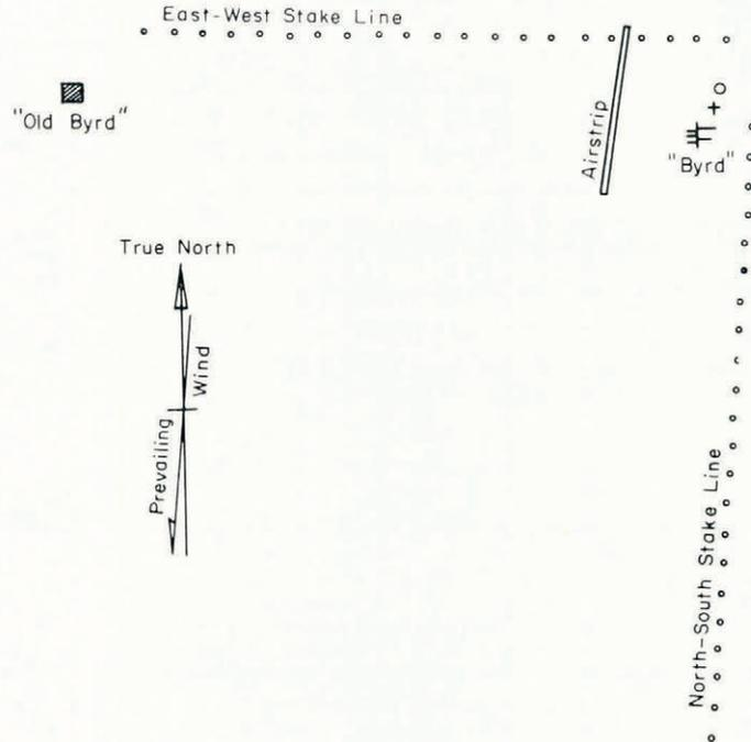
Fig. 1. Sketch map of "Byrd" station and environs showing locations of accumulation stake lines and radiometric sampling sites. Spacing between accumulation stakes is approximately 0.5 km. Location of samples used in this study is shown by a cross. Windom's (1969) sampling site is indicated by a circle.
