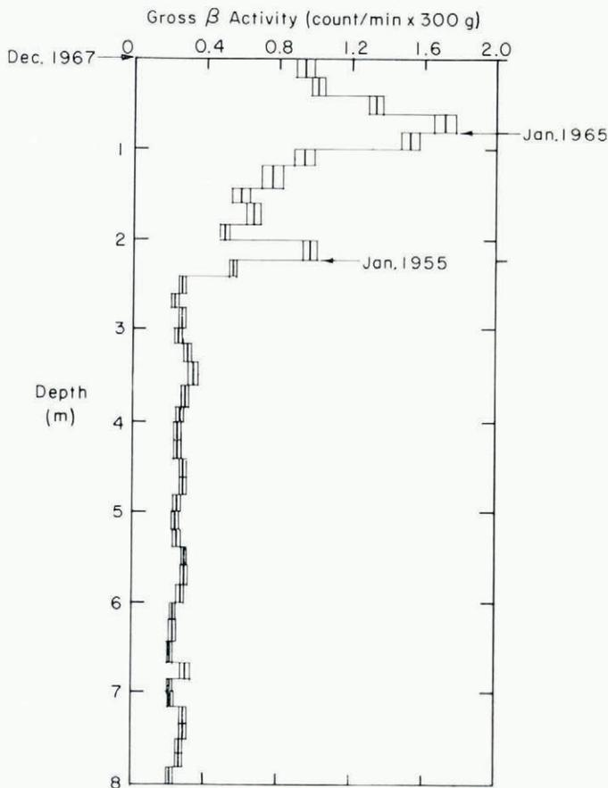
Fig. 3. Gross  $\beta$  activity in the firn at "Byrd" station. The  $\beta$  activity is expressed in counts per minute and per 300 g sample, without background correction. The error interval represents the standard deviation on the number of counts. The arrows show the positions of the  $\beta$ -activity maxima attributed respectively to January 1955 and January 1965.
