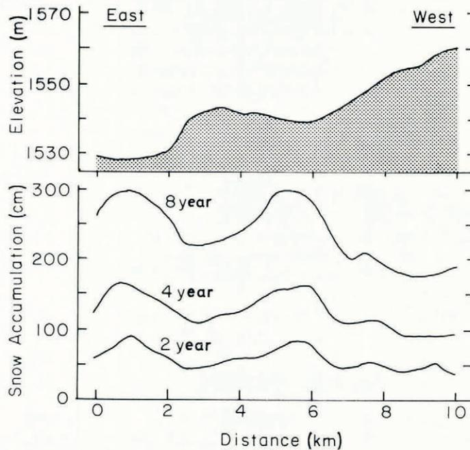
Fig. 2. Relationship of snow accumulation to undulating surface topography along the east-west stake line at "Byrd" station Antarctica. Surface depressions are accumulating 30–50% more snow than the exposed crests.
