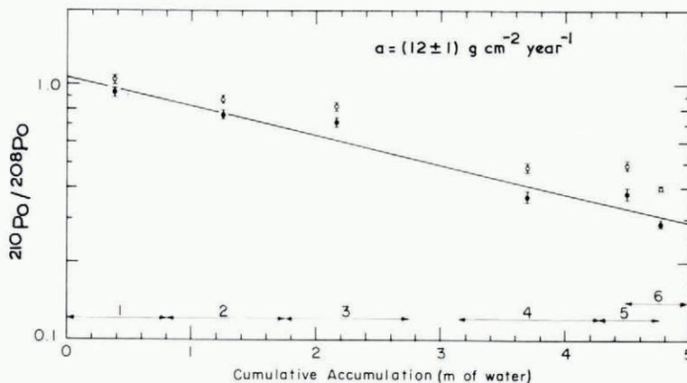
Fig. 4. Variation of the  $^{210}\text{Pb}$  activity in the firn as a function of depth in water equivalent.  $^{210}\text{Pb}$  activities are expressed relatively to the activity of the  $^{208}\text{Pb}$  tracer. Open circles represent uncorrected activity ratios. Dots represent activity ratios corrected for background. Error bars indicate the uncertainty due to counting statistics.
